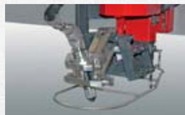
Optional 3D-Link for bevel cutting can be attached
